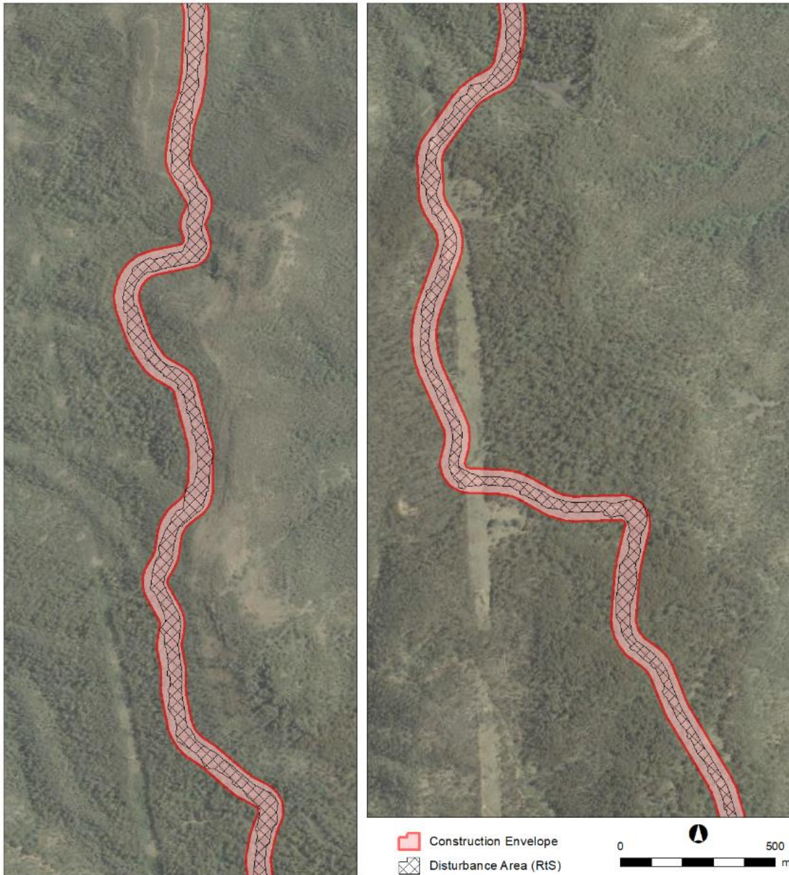
Figure 1-3: Disturbance area and construction envelope
