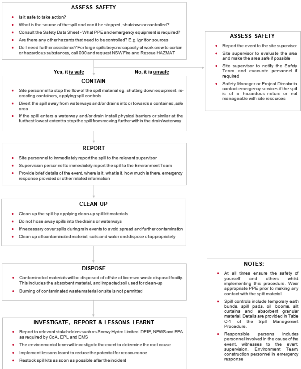
Figure C 1: Emergency Spill Response Flow Chart
