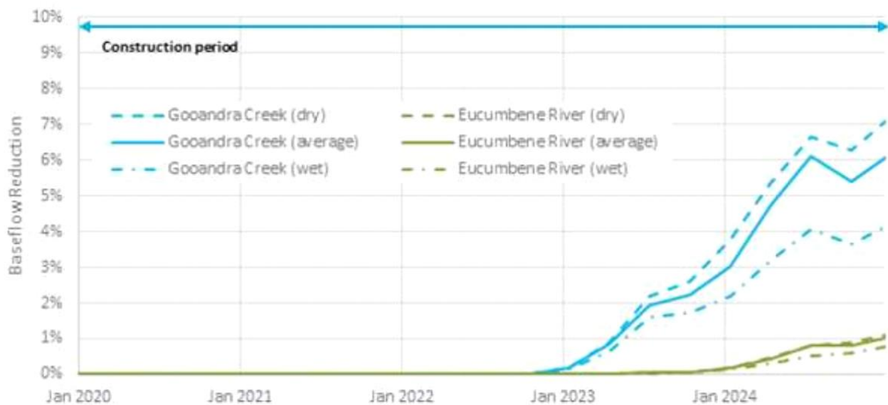
Figure 4-2: Baseflow reduction predicted by the groundwater model during project construction
