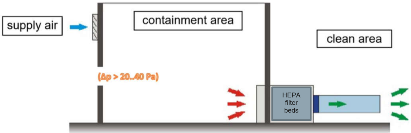
Figure 5-2: Tantangara containment shed principle of air supply, extraction and treatment.
