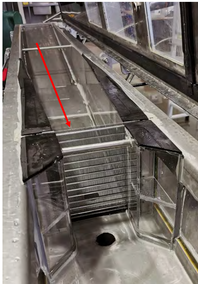
Figure 12: Top: schematic of the experimental flume with the tapered inlet modifications (orange). Bottom: Tapered inlet installed in the experimental flume, red arrow is direction of flow (Source: Doyle et al., 2023).
