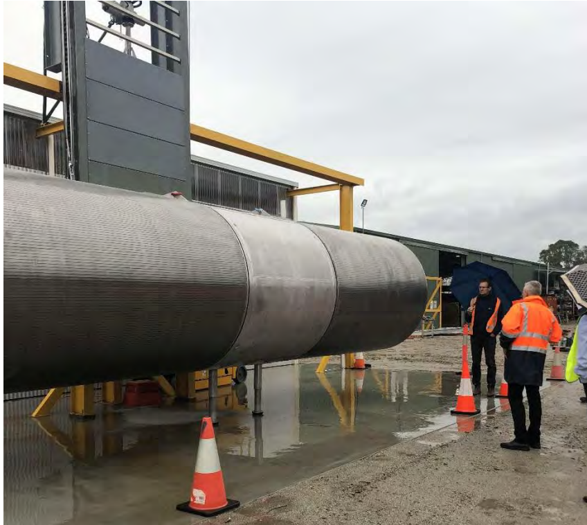
Figure 6: Example of cylindrical fine mesh wedge wire screen similar to that planned for Tantangara
