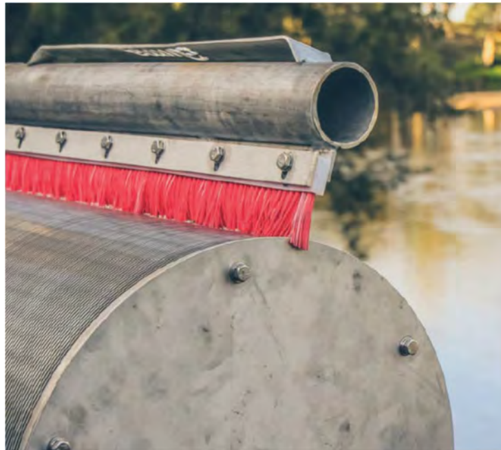
Figure 11: Example of brushes used in wedge wire screens (Source: NSW DPI, 2021 p.31)
