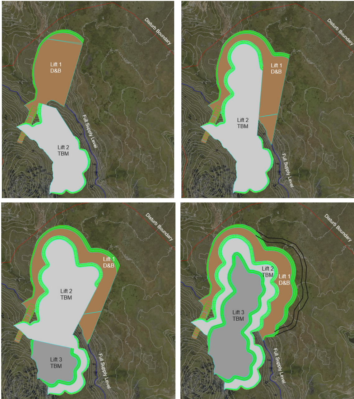
Figure 4-2 Indicative construction sequence, Tantangara PSE
