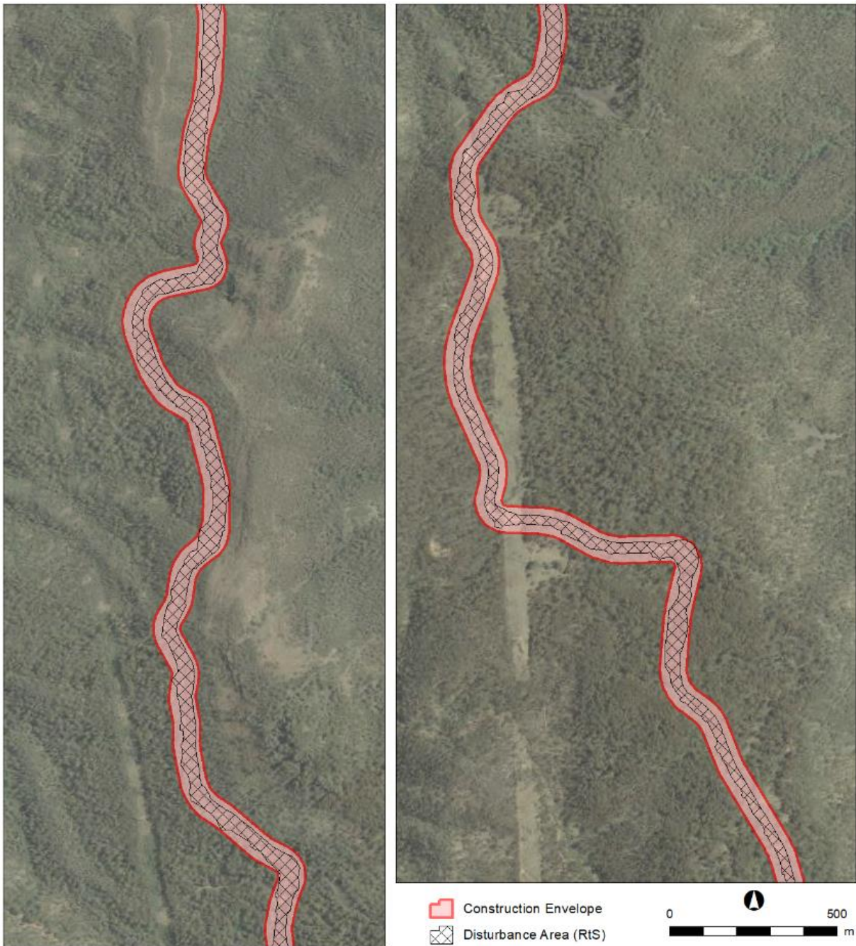
Figure 1-3: Disturbance area and construction envelope
