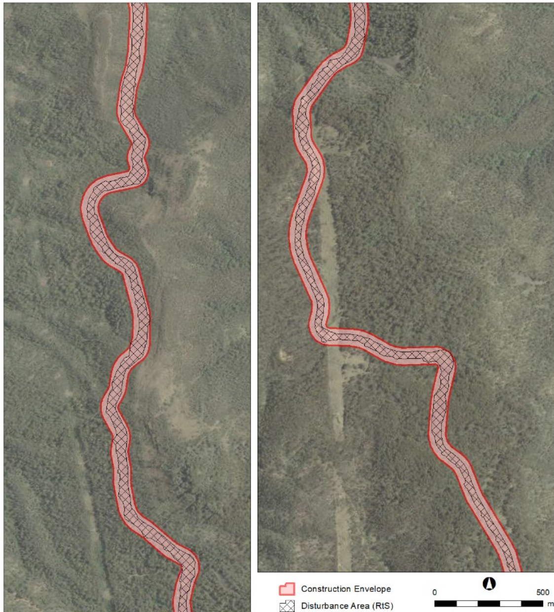
Figure 1-3: Disturbance area and construction envelope
